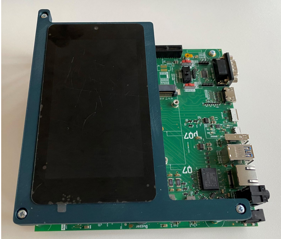
Fig. 1.9: Plug in the Haikou Video Demo on the Haikou carrier board
