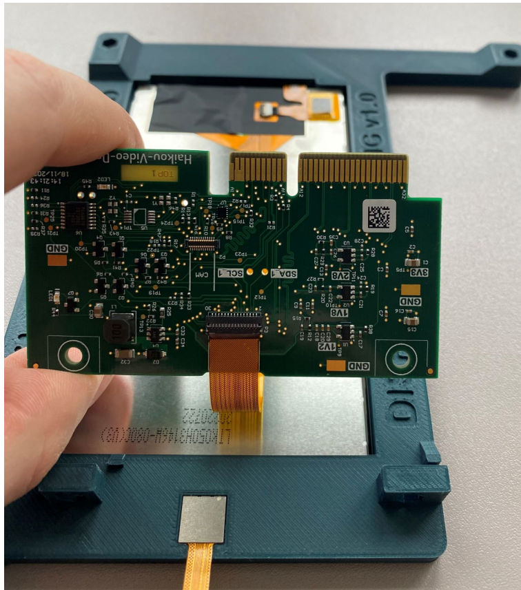
Fig. 1.3: Connecting flat-flex cable to the Haikou Video Demo PCB
